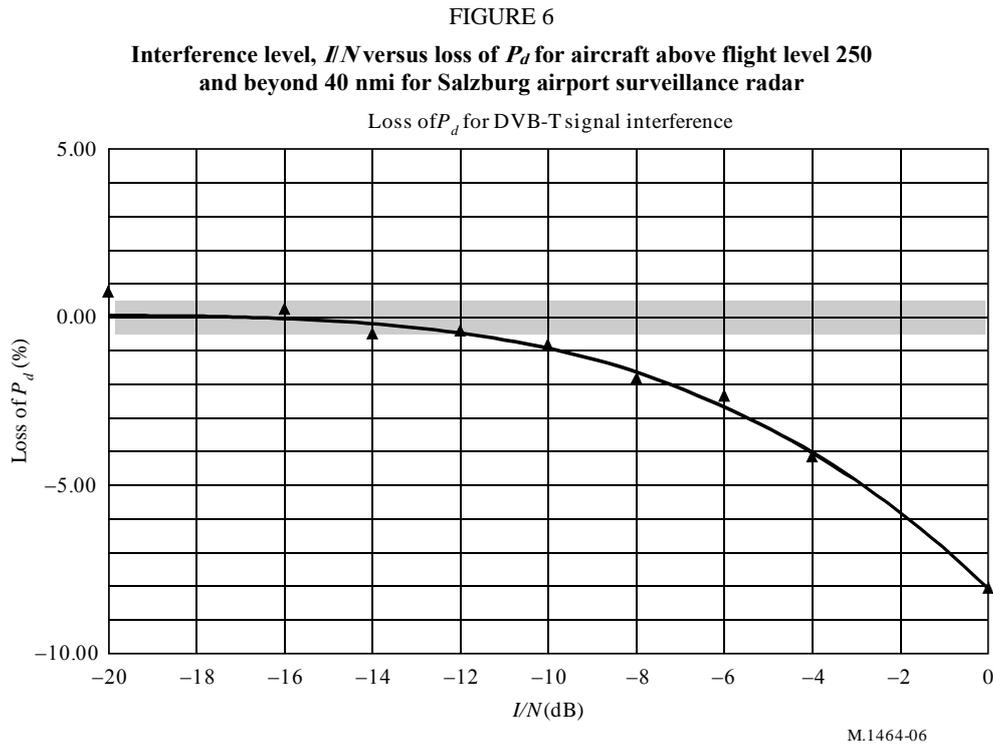
At  $I/N = -6$  dB there is already a loss of about 2.5% detection probability and at  $-10$  dB it is 0.8% which is still outside the error margin. The interpolation curve shows that the drop of  $P_d$  starts about  $-14$  dB and becomes significant above  $-10$  dB. Figure 7 shows the same data but as a function of  $\Delta S/N$  instead of  $I/N$ . The sensitivity of the  $P_d$  on the loss of  $S/N$  is about 3%/dB between 1% and 7% loss of  $P_d$ .
