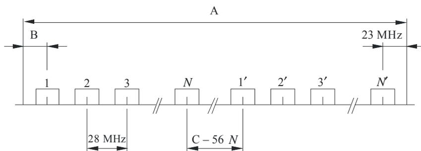
Pour la bande 14,4-15,35 GHz: A = 950 MHz, B = 17 MHz, C = 966 MHz
