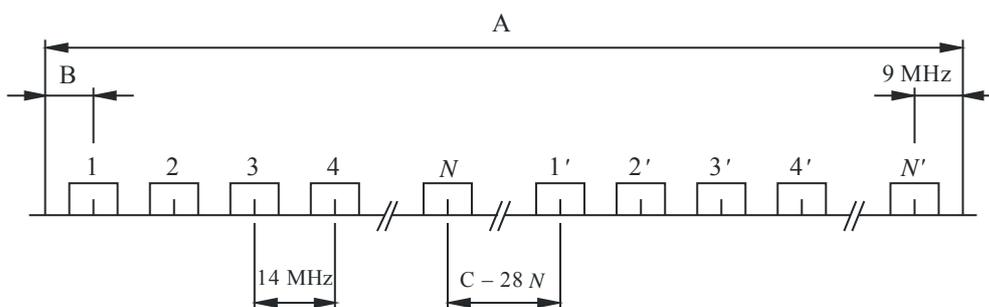
Pour la bande 14,4-15,35 GHz: A = 950 MHz, B = 17 MHz, C = 952 MHz
