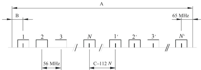
Pour la bande 14,4-15,35 GHz: A = 950 MHz, B = 31 MHz, C = 966 MHz
