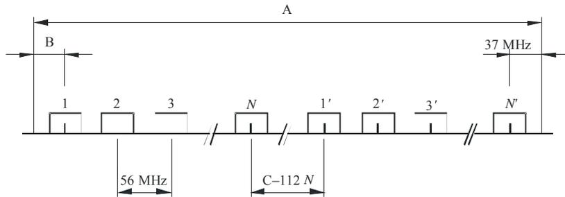
Pour la bande 14,4-15,35 GHz: A = 950 MHz, B = 31 MHz, C = 994 MHz
