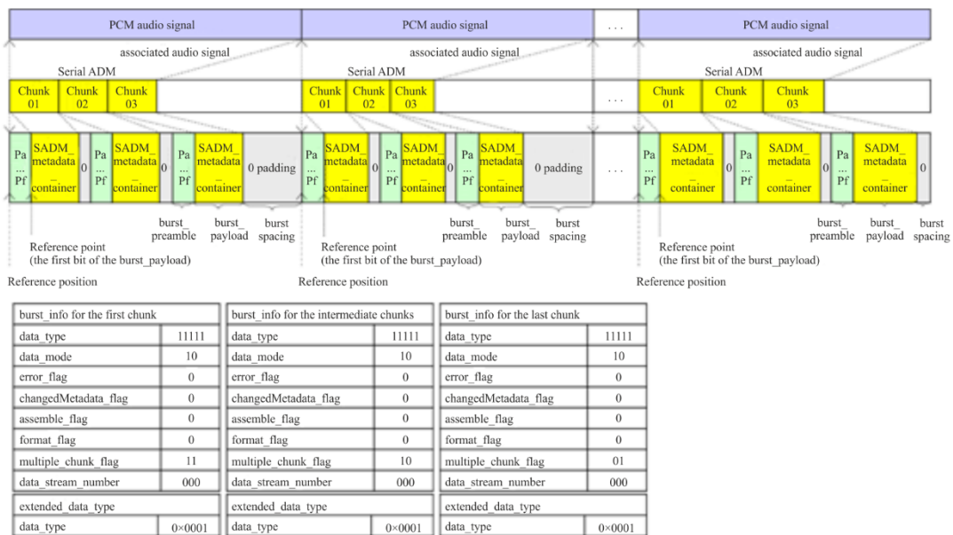
FIGURE 8 Structure of the data burst sequence for multiple chunks
