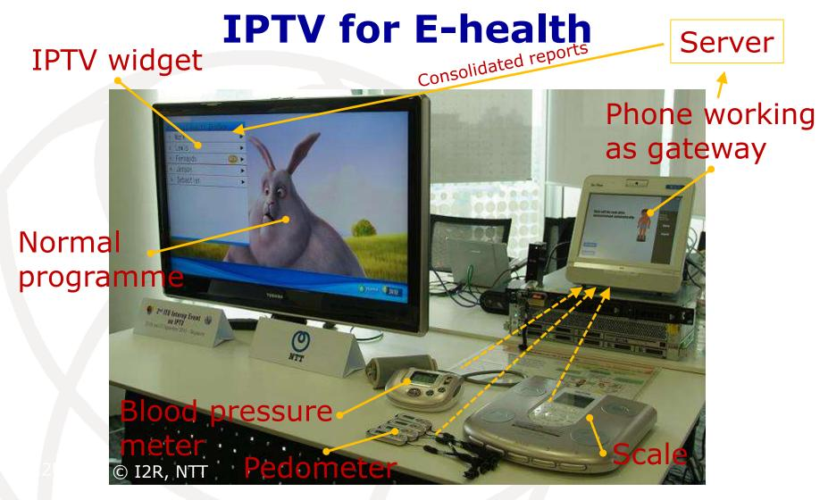
Widget implemented with LIME (ITU-T H.762) for e-health information collected from the user site, consolidated in the server backend and displayed on users' IPTV terminal device as a widget.
