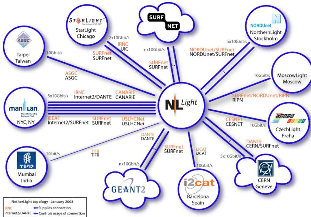
At its heart, NetherLight has a Nortel HDXc optical cross connect that interconnects multiple 10 Gbps optical wavelengths (or lambdas). This allows the interconnection of lightpaths from different national and international network facilities, including StarLight in the USA and the Global Lambda Integrated Facility (GLIF).
