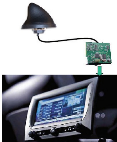
Figure 2: Example of a two-part solution for in-vehicle implementation of CALM
