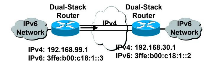
Configured tunnels require: Dual stack end points
