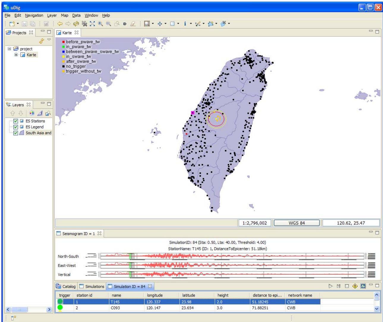
Fig. 9 Screenshot of GIS-based Visualiser and Topology Editor (showing simulation 84).
