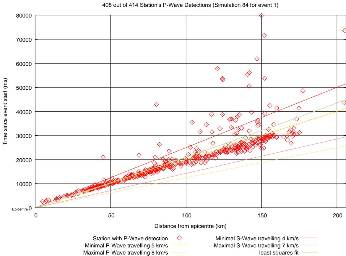
Fig. 8 Time-distance diagram of event detections for ChiChi earthquake (showing simulation 84).
