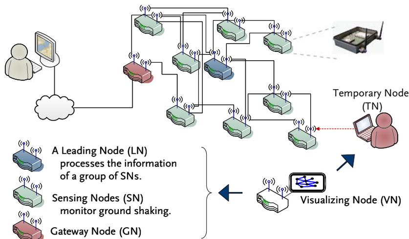
Fig. 1 A SOSEWIN example topology with typical nodes.
