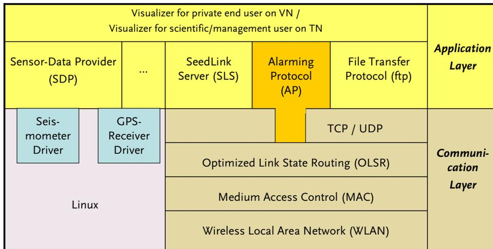
Fig. 3 The SOSEWIN software architecture.
