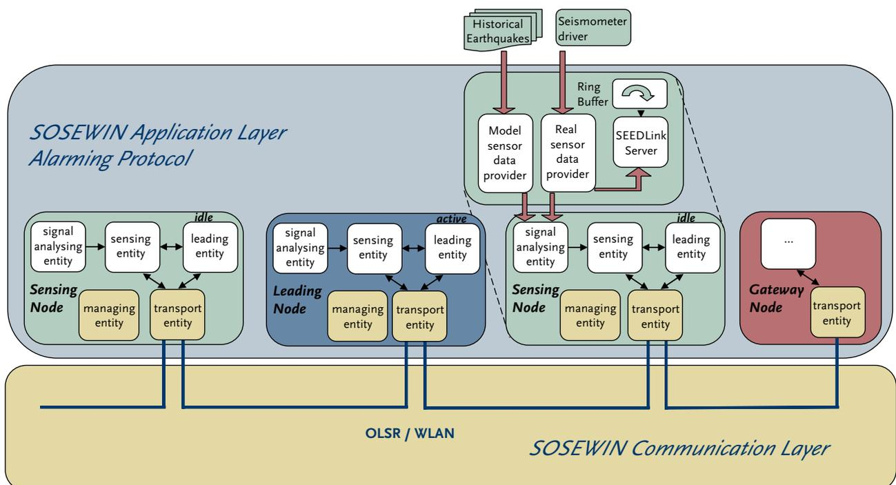
Fig. 4 Nodes and the associated protocol entities of the SOSEWIN Application Layer.
