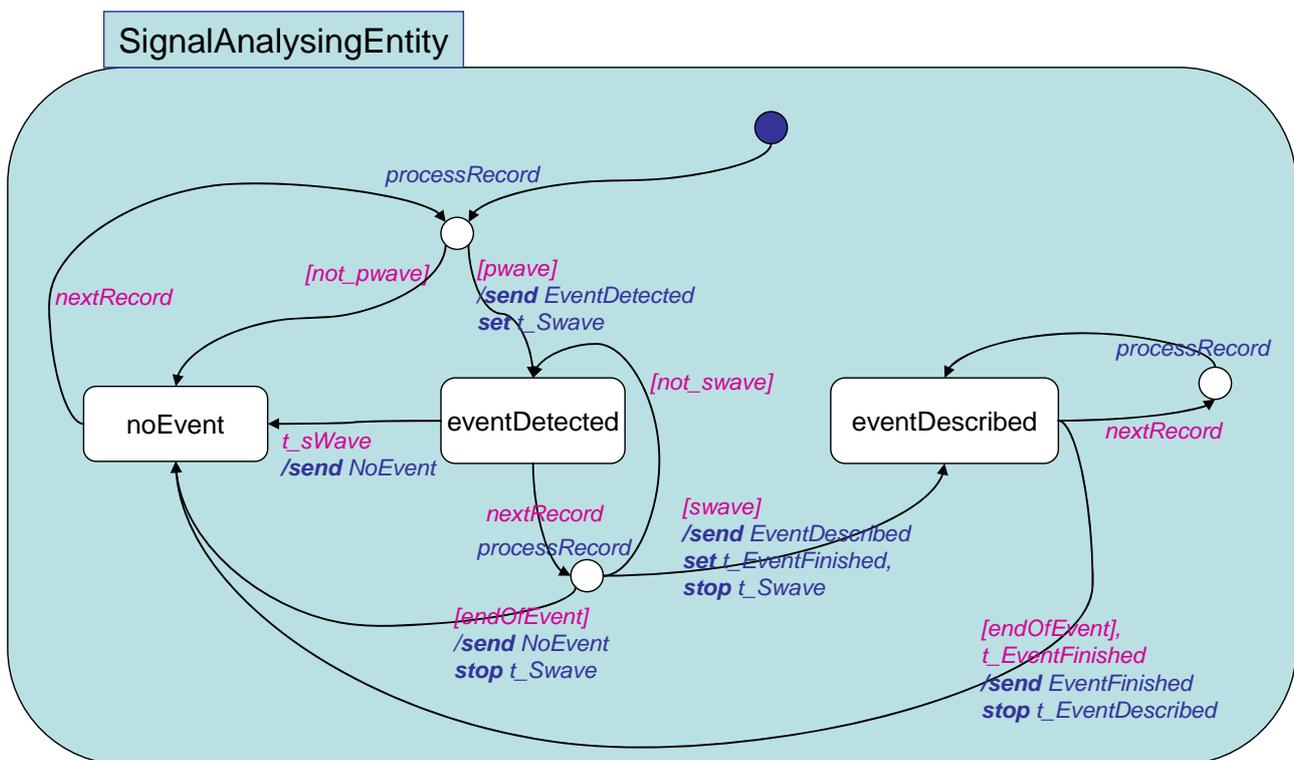
Fig. 6 Signal Analysing Entity as an UML State Machine.
