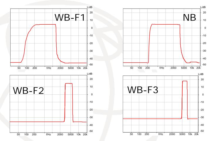
Filter chosen such that the measured echo loss with speech as an input signal is identical for all filters
