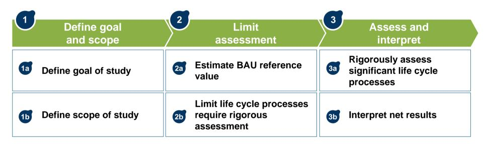
Methodology uses a Life Cycle Assessment (LCA) approach to guide the assessment of changes to an existing system resulting from the adoption of an ICT solution
