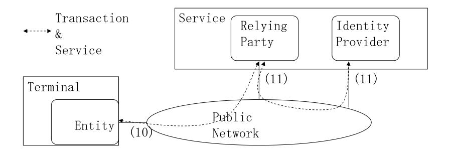
The terminal/end user equipment accesses to the public network via the User Network Interface UNI (10).
