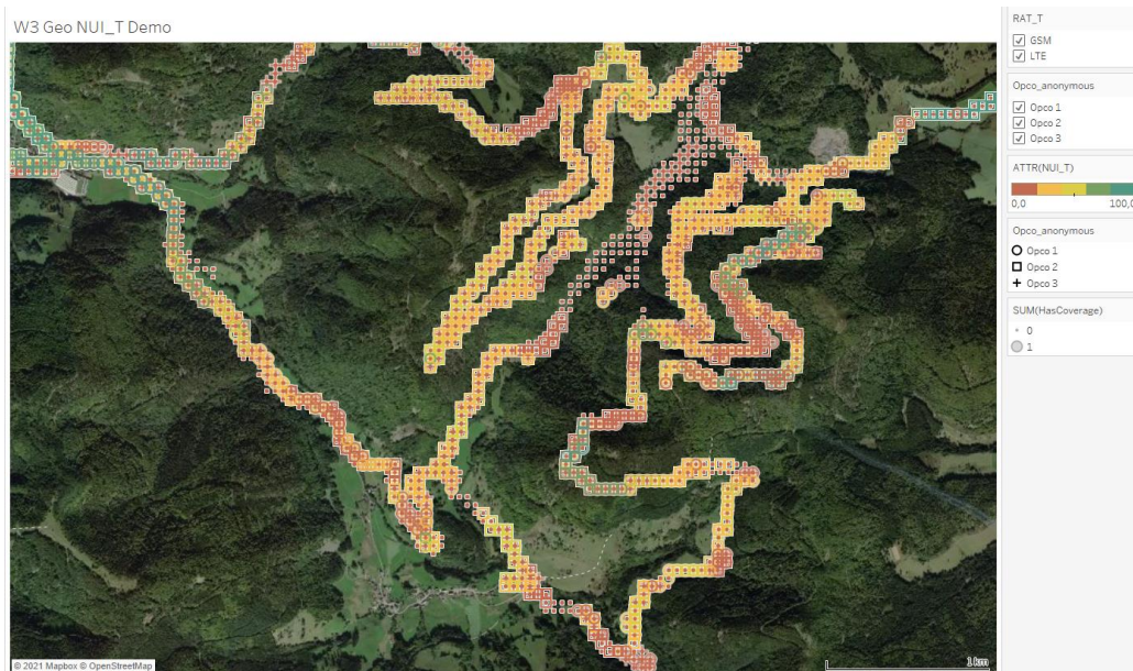
Figure 3 – Example of a tiled geo-visualization for NUI_T (color-coded) and three mobile networks. Symbol size according to a binarized version of NUI_T
