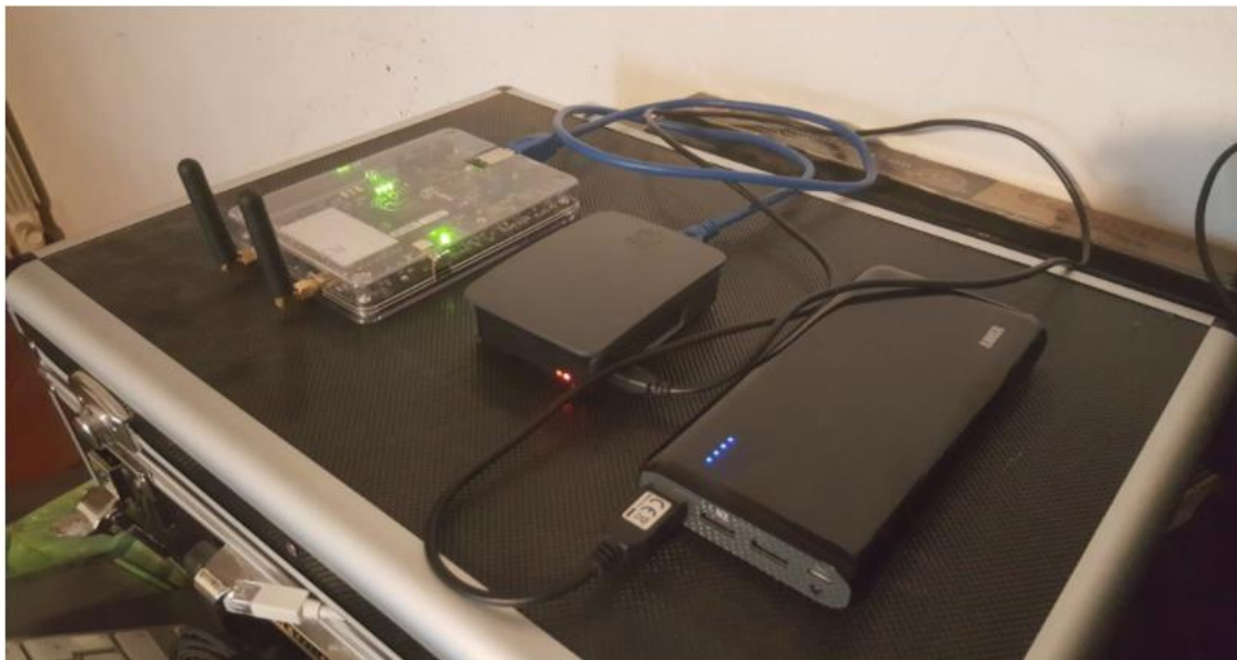
Figure 4 –A rudimentary MITM interception system based on commercial HW and open-source SW
