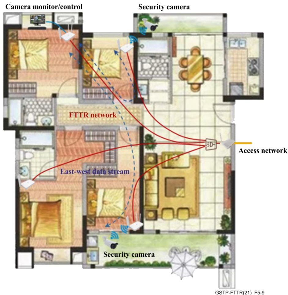
Figure 5-9 – Example of the East-west data stream (security camera)
