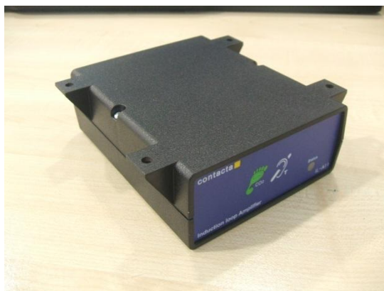
Figure 9 – Small-area hearing loop driver, typically installed under a counter
