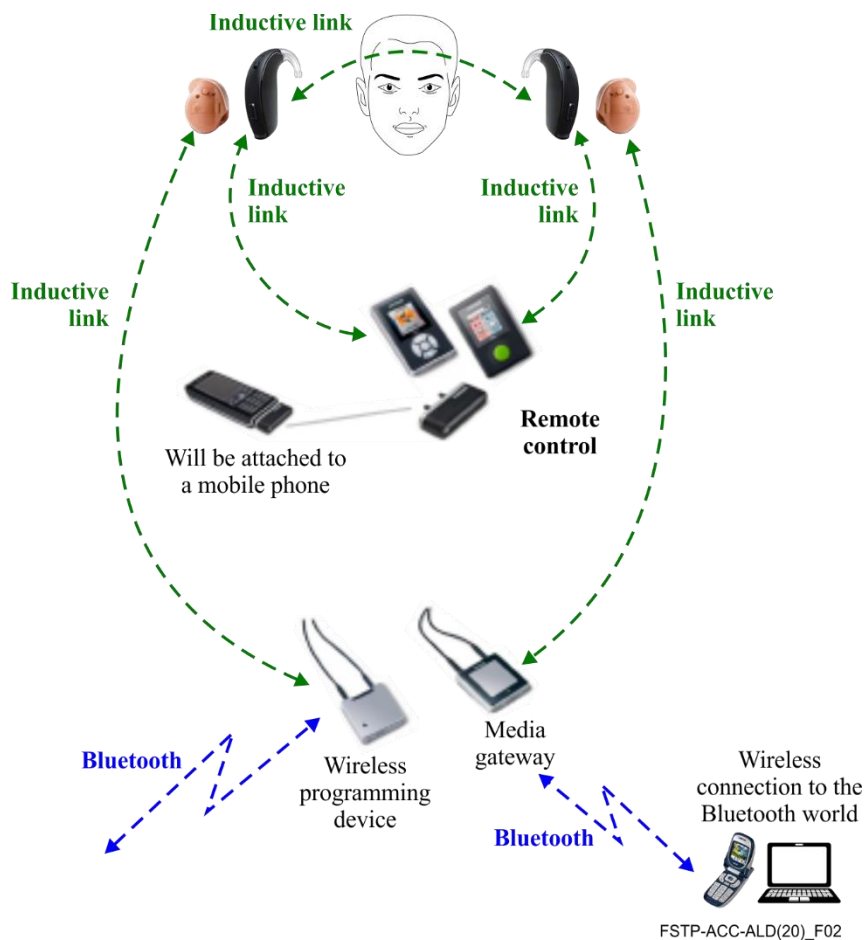
Figure 2 – Connection possibilities for ALDs
