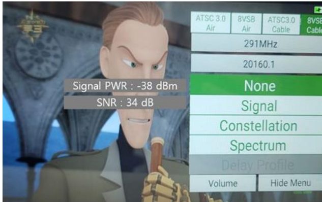
Figure 10 – An example of a remodulated ATSC 1.0 signal in an integrated-MATV system
