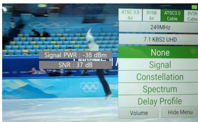
Figure 9 – An example of a remodulated ATSC 3.0 signal in an integrated-MATV system
