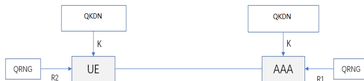
Figure 12-9 – Secondary authentication protocol based on quantum security
