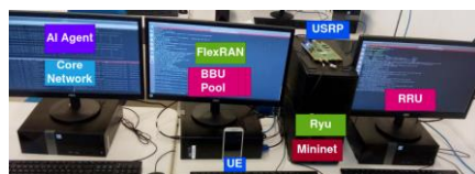
Figure 8 – Testbed working at LASSE – UFPA lab using a C-RAN architecture
