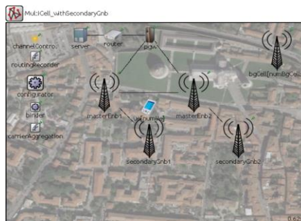
Figure 15 – NED file for MultiCell_withSecondaryGnb
