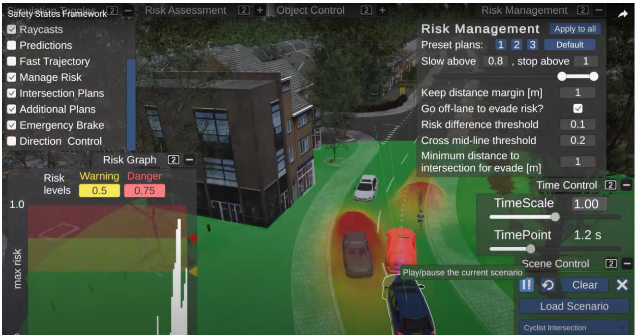
Figure 19 – Remote monitoring and risk assessment with the SSF: the ego vehicle stops the overtaking manoeuvre of the cyclist based on the forecasted risk (grey and orange ghost cars). It passed the maximum risk threshold. It remains behind the cyclist because cars could enter the crossing from the left road at the intersection
