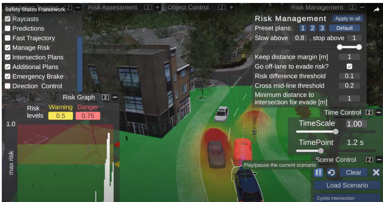
Figure 7 – Remote monitoring and risk assessment with the SSF: the ego vehicle stops the overtaking manoeuvre of the cyclist based on the forecasted risk (grey and orange ghost cars). It passed the maximum risk threshold. It remains behind the cyclist because cars could enter the crossing from the left road at the intersection
