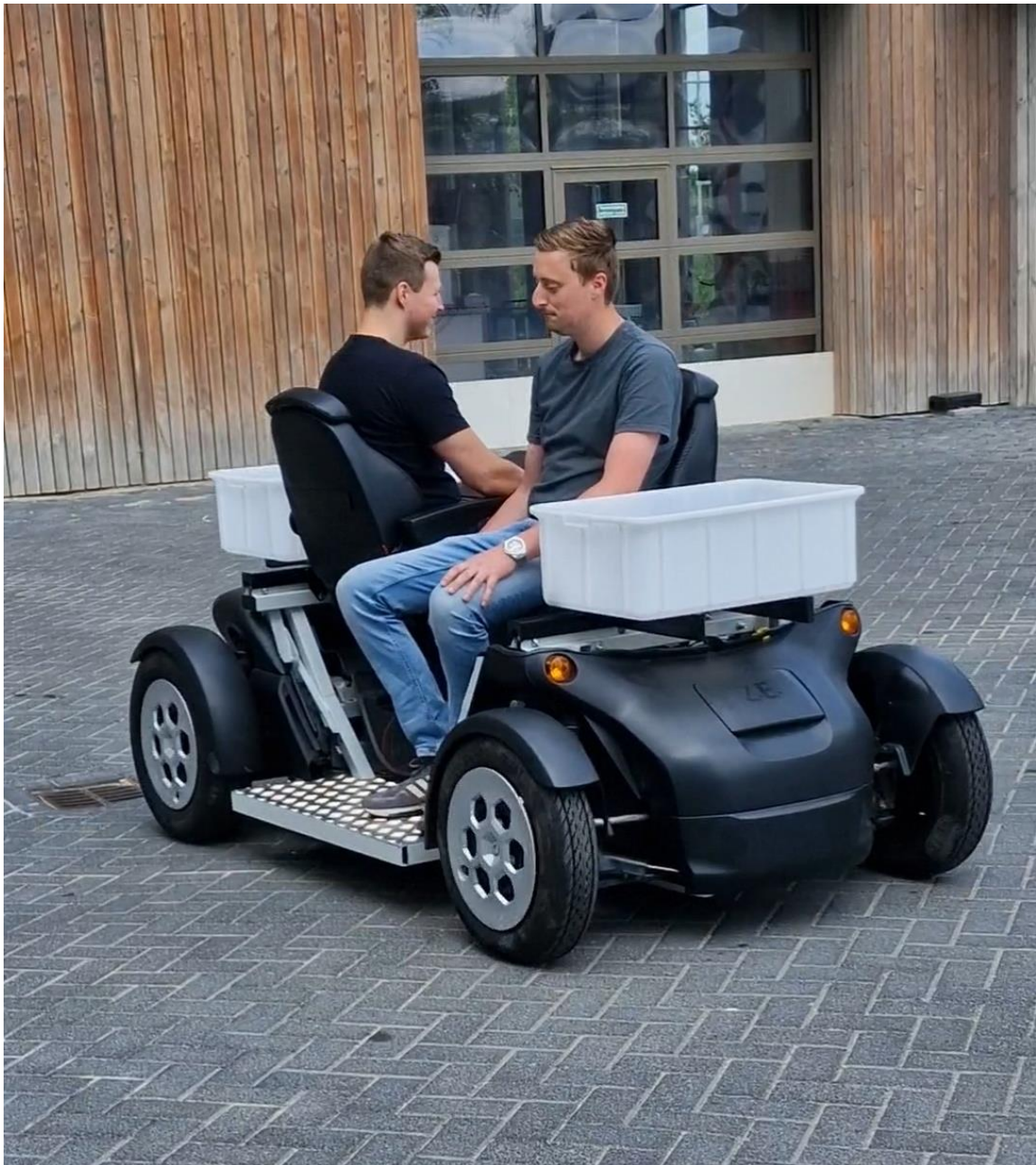
Figure 2 – The COLUMBUSS multipurpose microbus with exchangeable modules for transporting people and goods
