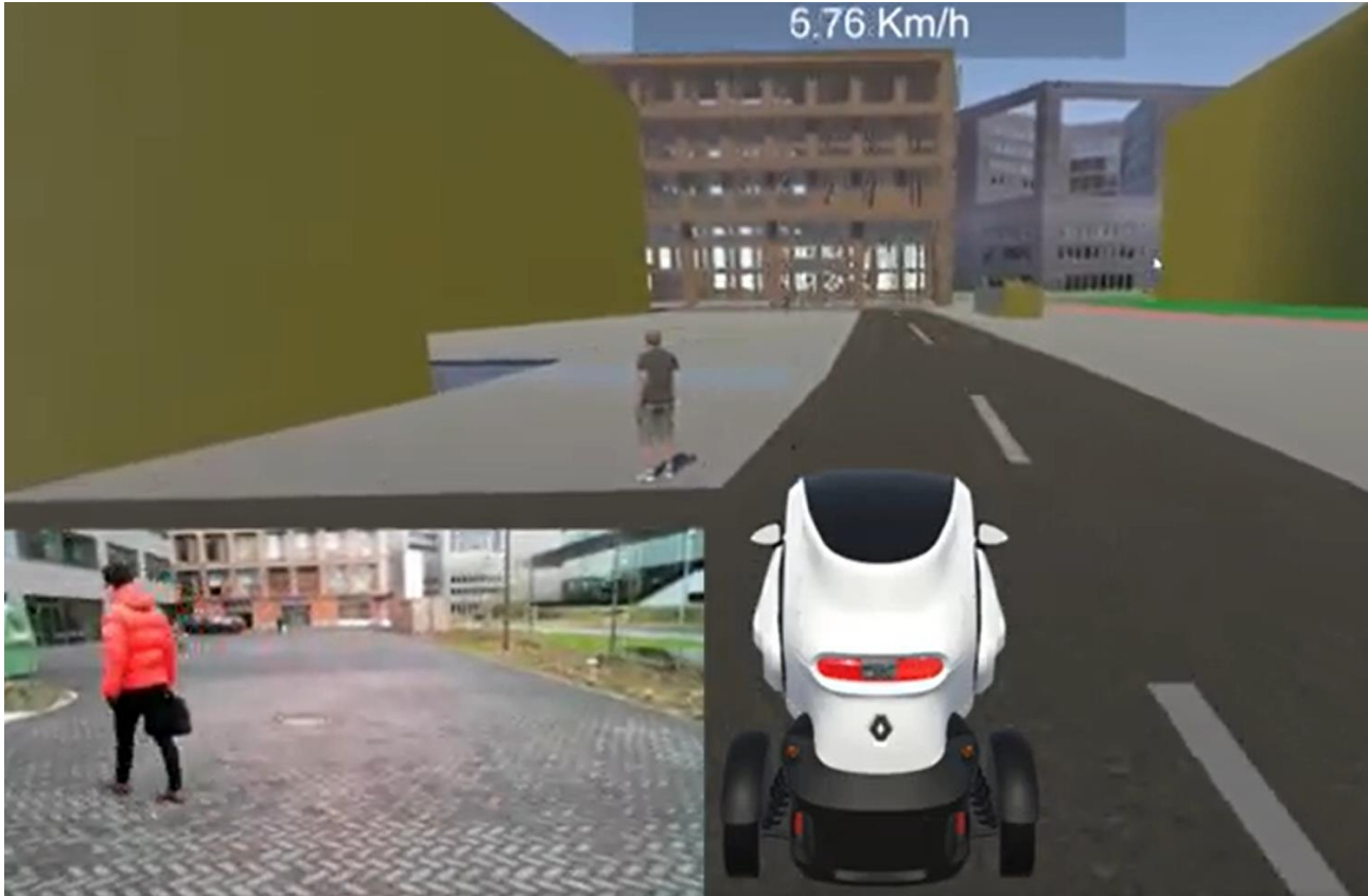
Figure 16 – Synchronized Digital Twin driving 6.76 km/h with a Renault Twizy ego vehicle: ODD is constructed with information from OpenStreetMaps and radar (pedestrian)
