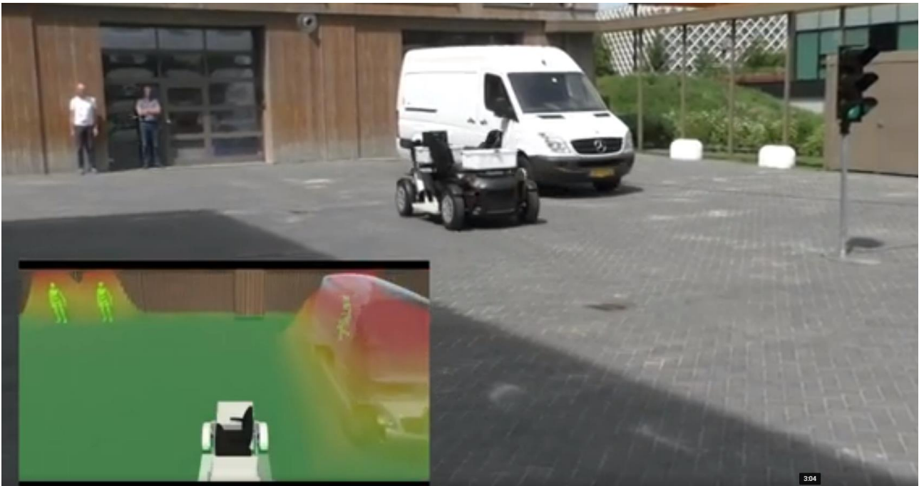
Figure 17 – MPV slows down for invisible pedestrian coming from behind the parked van, using the AI in the synchronized DT
