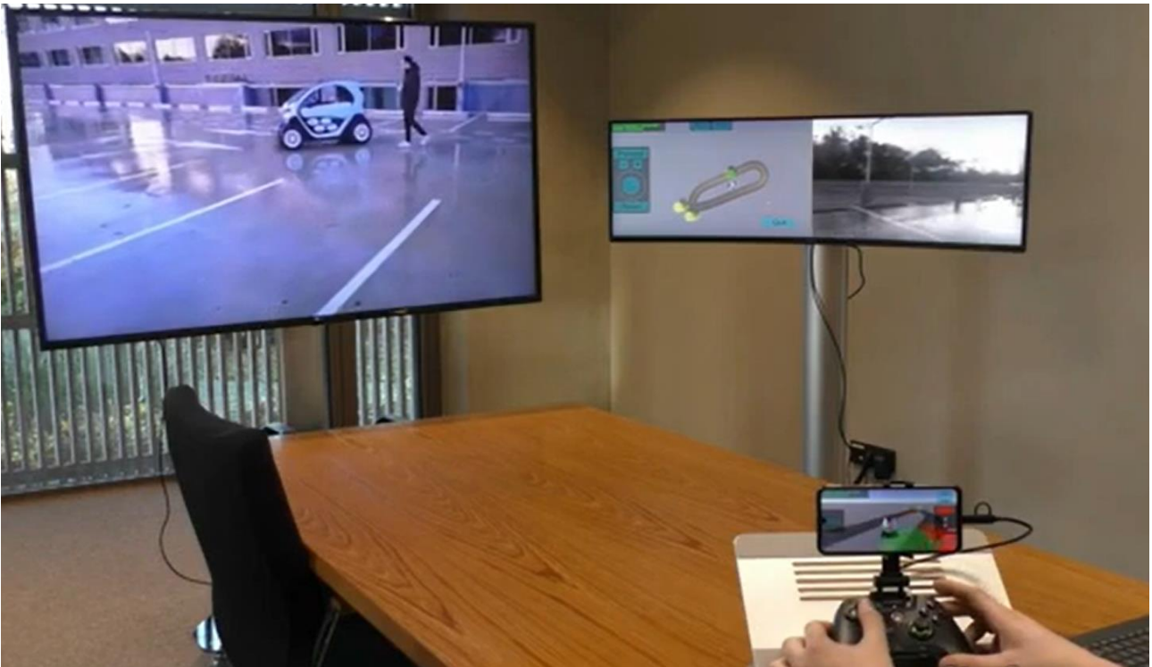
Figure 18 – Remote control in a 4G network. The DT runs remotely on a mobile phone
