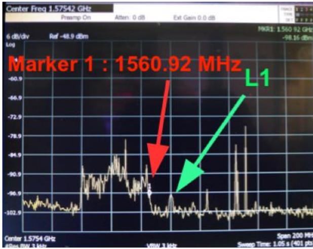
**Fig. 9** – Typical spectrum observed from end of January 2019 onwards. The center frequency is L1, the span is 200 MHz. Marker 1 highlights the threshold where the power received from the jamming signal is already surpassing the GNSS main lobe power inside the L1-band.
