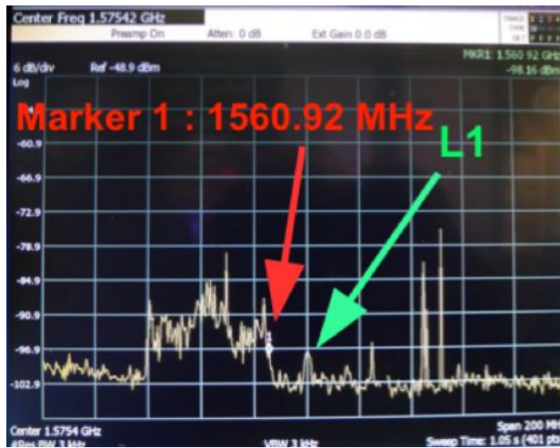
Fig. 9 – Typical spectrum observed from end of January 2019 onwards. The center frequency is L1, the span is 200 MHz. Marker 1 highlights the threshold where the power received from the jamming signal is already surpassing the GNSS main lobe power inside the L1-band.
