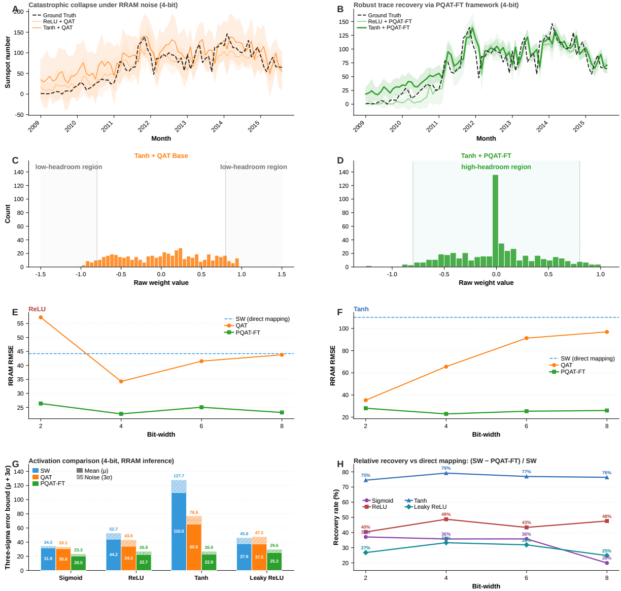
Figure 2 – Behavioral simulation under the aihwkit device-level noise model (50-trial Monte Carlo at inference with state-independent programming noise; additive Gaussian \sigma_n = 0.1 is injected only during noise-aware fine-tuning). (a)–(b) First 80 months of the 132-month test horizon. (a) QAT 4-bit baselines under RRAM noise: catastrophic prediction collapse with peak-to-peak deviations exceeding \pm 50\% for both ReLU and Tanh. (b) PQAT-FT 4-bit: robust trace recovery with tight trajectory bundling for both activations. (c)–(d) Tanh raw weight histograms: QAT 4-bit (c) spreads raw weights across a wide range, which can enlarge pre-activation magnitudes and thus increase the likelihood of saturation, whereas PQAT-FT 4-bit (d) concentrates them near zero through sparse regularization, leaving a physical conductance margin in the high headroom region. (e)–(f) Bit width scaling (2/4/6/8-bit) of RRAM RMSE for ReLU (e) and Tanh (f), comparing SW, QAT, and PQAT-FT. (g) Three-sigma error bound ( \mu + 3\sigma ) across four activations at 4-bit. (h) Relative recovery of PQAT-FT over direct floating-point mapping, (RMSE_{SW} - RMSE_{FT})/RMSE_{SW} , across activations and bit widths. The \mu + 3\sigma and relative-recovery percentages are derived from unrounded Monte-Carlo statistics.
