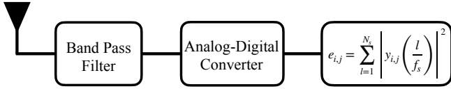
Figure 2 – Block diagram of the conventional ED technique [20].
