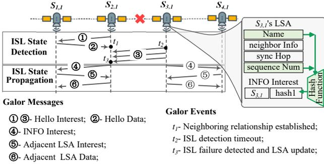
Fig. 3 – Illustration of routing mechanism in GALOR.
