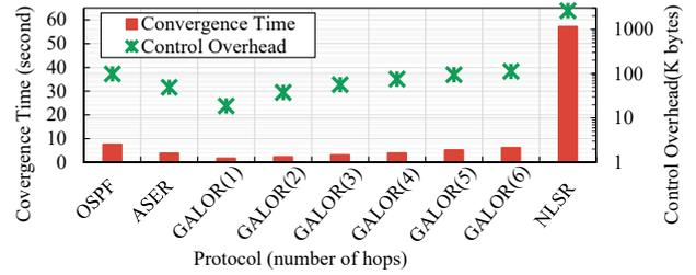
**Fig. 5** – Convergence time and control overhead achieved by OSPF, ASER, NLSR and GALOR( $k$ ), where  $k$  represents the number of synchronization hops.
