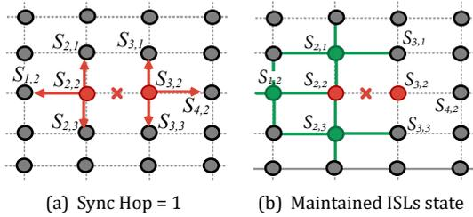
Fig. 4 – ISL state synchronization in GALOR within limited hops.
