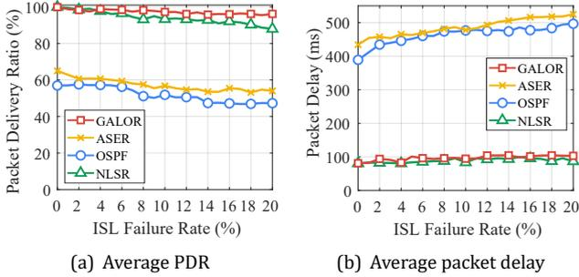
**Fig. 8** – Performance under different ISL failure rates in point-to-point traffic pattern (U8P1).
