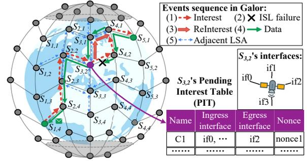
Fig. 2 - Illustration of content retrieval in GALOR. “intf” stands for a physical interface in the satellite.
