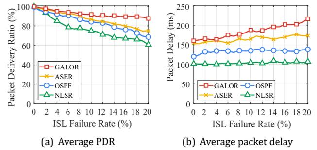
Fig. 7 – Performance under different ISL failure rates in point-to-point traffic pattern (U8P8).
