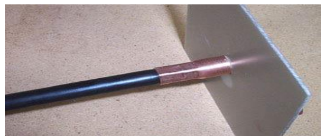
Fig. 6 – The copper pipe crimped onto the coax
