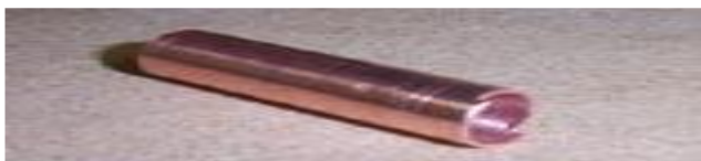
Fig. 1 – 50mm copper pipe with 2mm notch cut off
