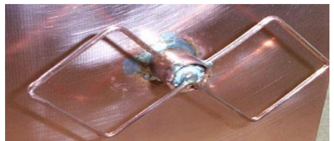
Fig. 5 – The complete bi-quad antenna with coaxial cable connected
