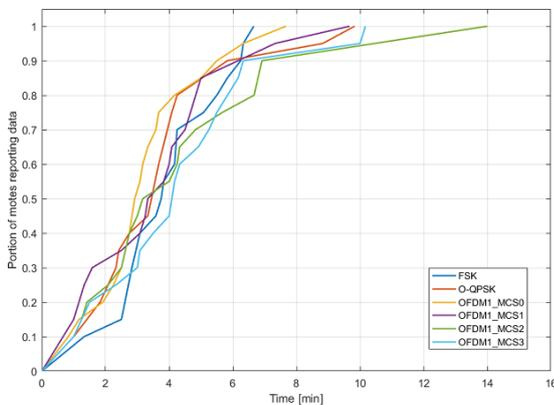
**Fig. 6** – The network formation time for the tested PHYs: 6 min for FSK, 9 min for O-QPSK, 7 min for OFDM1-MCS0, 9 min for OFDM1-MCS1, 14 min for OFDM1-MCS2, and 10 min for OFDM1-MCS3.
