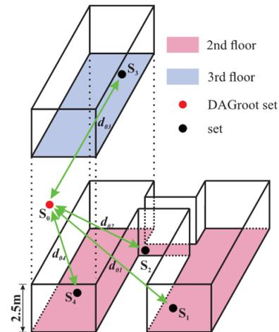
Fig. 4 – Experimental TestBed: Positions of sets across two floors at the premises of Faculty of Electrical Engineering.
