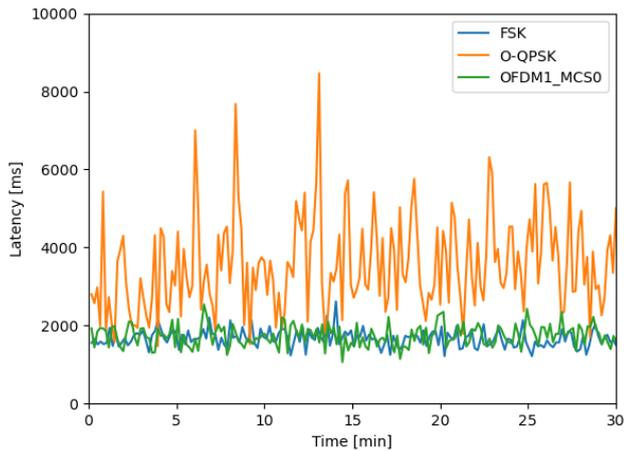
**Fig. 8** – The latency for O-QPSK 2.4 GHz, FSK 868 MHz and OFDM1-0 868 MHz PHYs.
