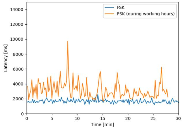
**Fig. 13** – The latency of the FSK network under two different scenarios: during and after working hours.
