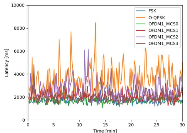
**Fig. 7** – The latency for the tested PHY networks.
