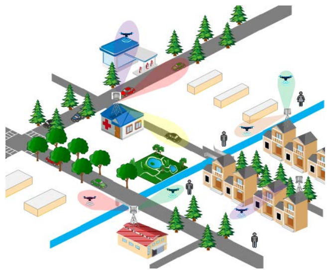
Fig. 2 – Beamforming from BS to both vehicles and drones.
