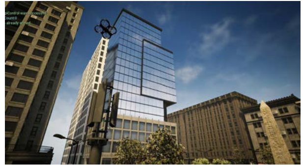
Fig. 3 – Scene from an INLOOP CAVIAR simulation in which a drone is served by a BS and RL is used for beam selection and for determining the drone trajectory.
