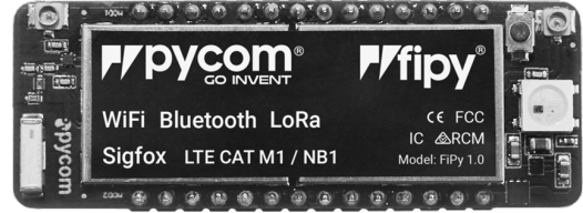
Fig. 2 – FiPy board from Pycom [18].
