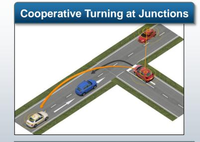
Based on notifications of intended turning, interested vehicles exchange info to coordinate right of way and transit maneuvers with increased time spans
