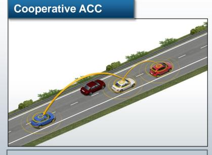
Rx vehicles analyze CACC status of tx vehicle/infra to modify communications & automation behavior (reduce gap/improve response to speed variations of preceding vehicle)
