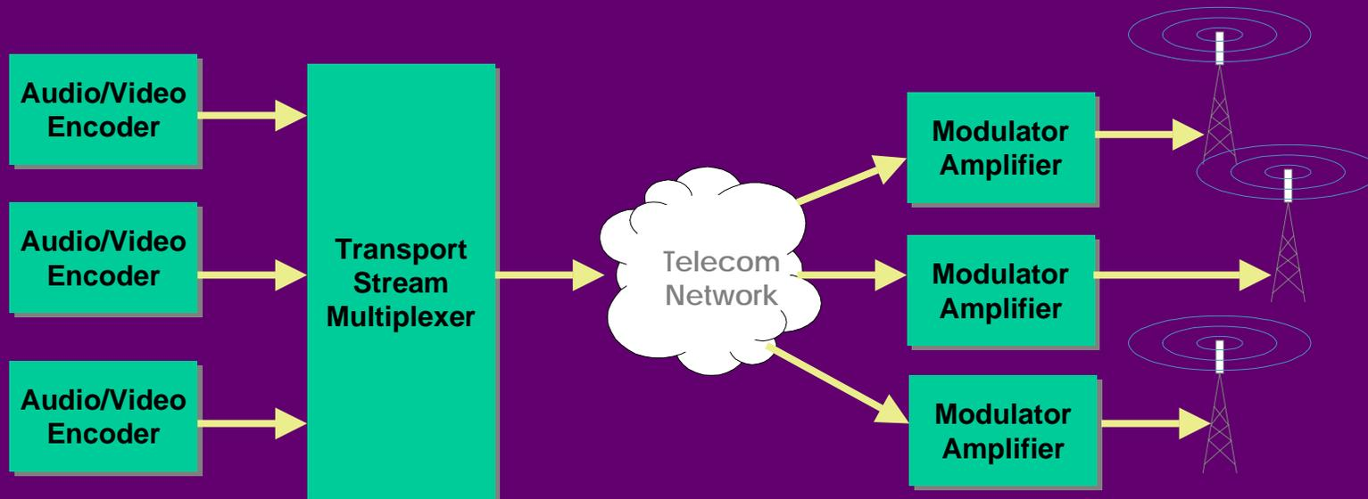
In a DVB-T structure several TV and Radio programs can share a common transmitter network
