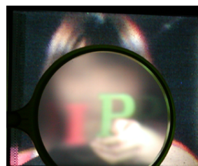
(c) Projected image on diffuser set 40mm away from lens array.
