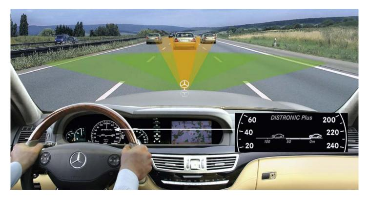
Long Range Radar sensors and Short Range Radar sensors observe the lane in front of the vehicle.
