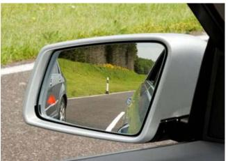
**Short Range Radar** sensors in the rear bumper observe the vehicle's blind spots. The driver is assisted in three stages:
