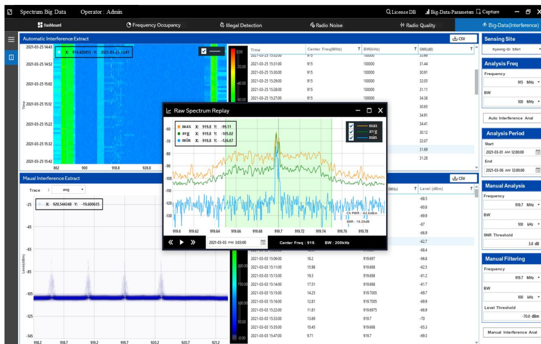
FIGURE 7 Spectrum monitoring with local processing for illegal transmission and interference detection
