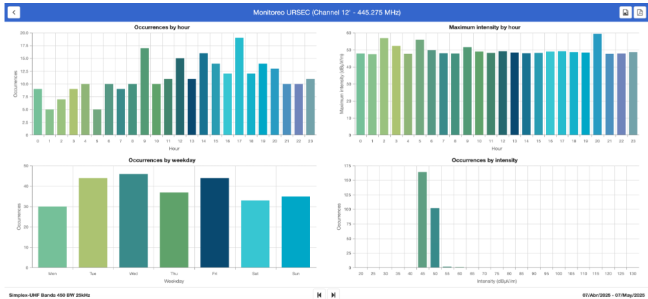
FIGURE A3-6 Online display of historical results for a channel in the UHF band
