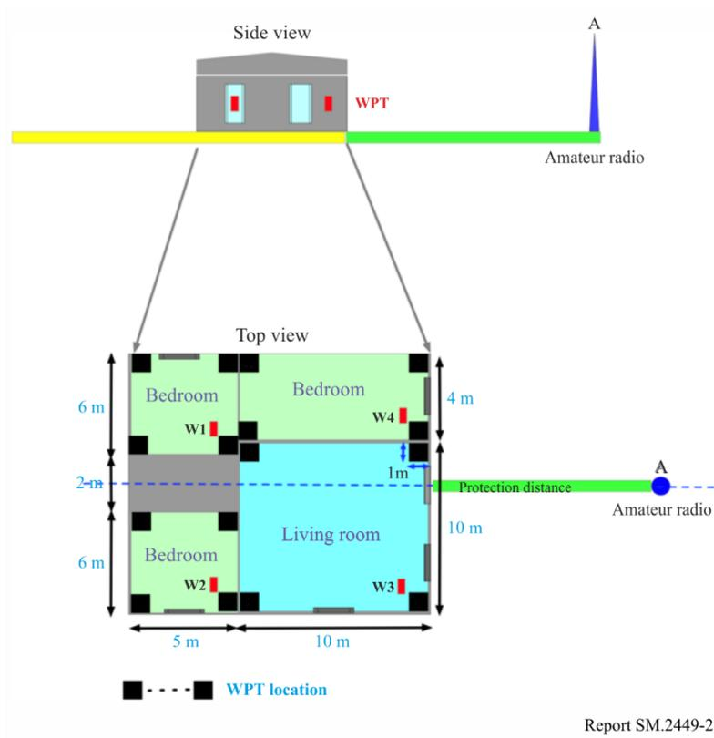
To simulate different building materials, the building entry loss for both wooden and concrete walls were assessed to determine the protection distance. The values are included in Table 11.
