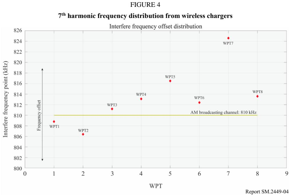
The tested impact to both broadcasting receivers (AM1 and AM2) from each wireless charger is summarized in the following Figures and Tables. The Figures use three impact levels (see Table 2) to assess the level of audible noise each wireless charger caused to the AM receivers to plot the best and worst audible interference, level 1 being intolerable and level 3 being inaudible. The impact level decreases as the distances increases between the wireless charger and the AM receiver.
