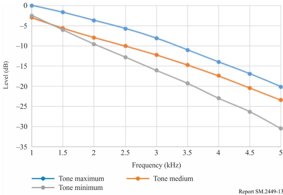
The behaviour of the Receiver 1 tone control is rather strange; it seems to have more of an effect on the overall level than on the treble response, which is (presumably) largely determined by the IF filters. For the purpose of the interference tests, the control should be set to maximum, to keep the response about right at 2 kHz. The response at 5 kHz is less important, since the interferer would be deliberately placed at about 2 kHz offset from the wanted carrier to represent the worst case.
