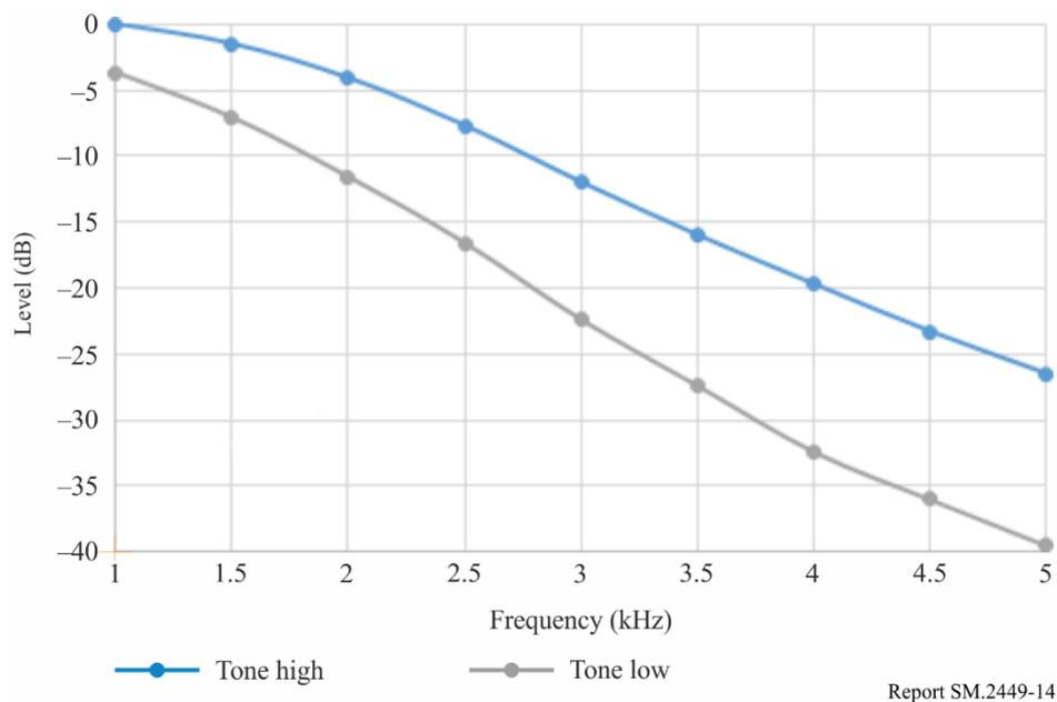
The action of the tone control (switch) is drastic indeed. It is clear that any testing should be carried out with the switch in the ‘High’ position – there is nothing intermediate between ‘High’ and
