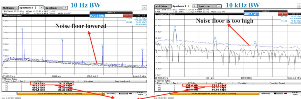
The AM receiver signal bandwidth setting is shown in Fig. 8. Based on the 1 dB difference, 10 Hz was also used for the AM receivers.
