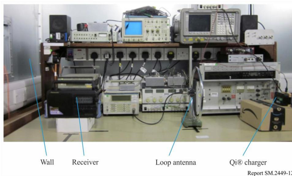
The ferrite antenna in the receiver and the charger were arranged to be on the perpendicular axis of the loop antenna. For the tests the receiver was 0.5 m from the wall, the loop antenna 1.0 m and the charger 1.2 m.
