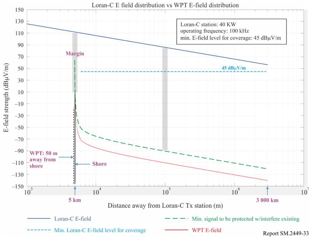
Figure 34 is the consolidated data for different aggregate cases. The Figure depicts the E-field signal levels of 100 and 10 000 active WPT devices operating simultaneously. When 10 000 active WPT devices are operating at 100 kHz simultaneously, there is a 3.88 dB margin between the signal to be protected (66 dBµV/m for 100 devices and 106.12 dBµV/m for 10 000 devices) and the E-field strength of the Loran-C transmitter, which is greater than 110 dBµV/m at the shore.
