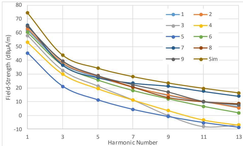
In general, the level of harmonic  $n$  for each device obeys the expected  $(1/n)$  law. (The plots run parallel to the ideal ‘Sim’ figures.) This confirms that the tuned circuit is indeed driven by a square wave. As pointed out in Section 4, the  $1/n$  relationship does not apply to the fundamental component, since the tuned circuit incorporating the coupling inductor is then close to resonance.
