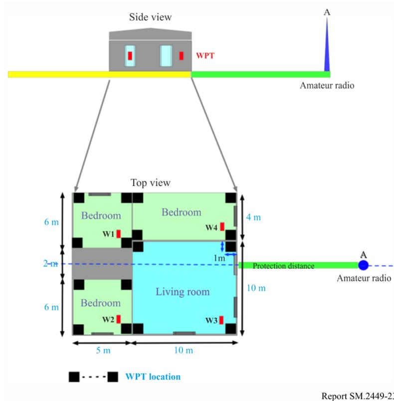
To simulate different building materials, the building entry loss for both wooden and concrete walls were assessed to determine the protection distance. The values are included in Table 13.
