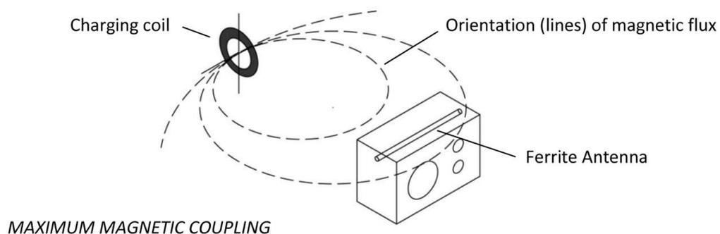
With the ability to move and rotate both the charging coil and the receiver in a three-dimensional space there is scope for the magnetic coupling between the coil and the receiver to be anything between the maximum and, potentially, none.
