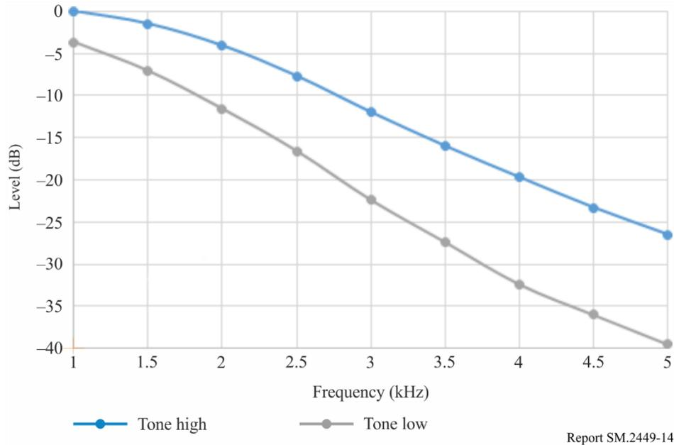
The action of the tone control (switch) is drastic indeed. It is clear that any testing should be carried out with the switch in the ‘High’ position – there is nothing intermediate between ‘High’ and ‘Low’ – where the modulation response is a good match to that of the Recommendation ITU-R BS.703 reference receiver.
