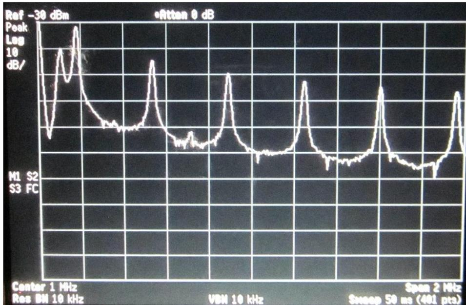
An interpretation of the spectrum is that the device spends most of its time at 175 kHz, but momentarily tries 100 kHz (its normal operating frequency). The audible effect on an AM receiver is a ‘double thump’ corresponding to the start and finish of the burst. This is as expected: the sudden changes in carrier level give rise to low-frequency transients.
