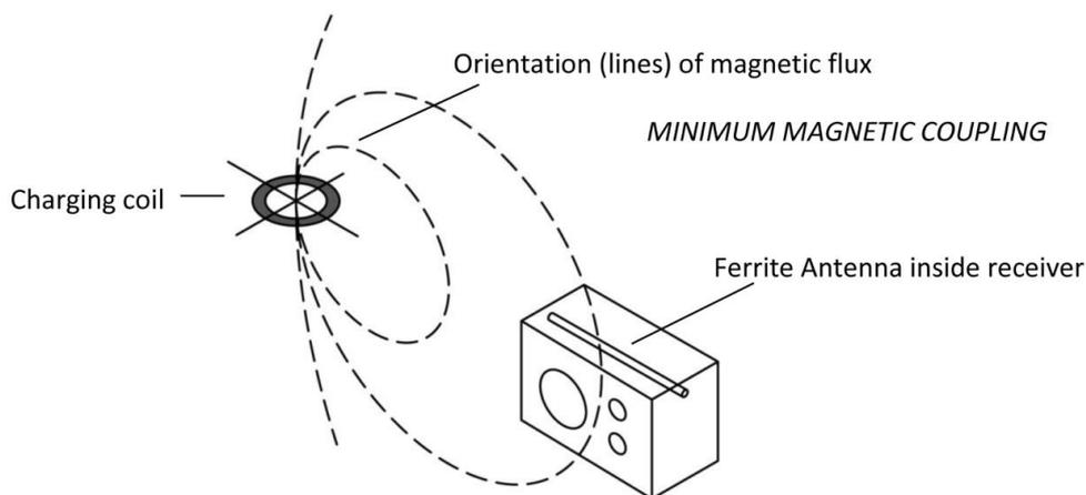
By turning the receiver through 90 degrees horizontally, and the charging coil through 90 degrees vertically, as shown in Fig. 8, the magnetic coupling and hence the level of the interference will be considerably increased; in fact maximised. The orientation of the magnetic flux inside the receiver will be parallel with the axis of the ferrite antenna.
