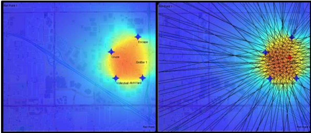
Figure 15 (left) shows the expected geolocation coverage area (assuming correlation of up to four sensor pairs) and the hyperbolic lines to the emitter location. The right figure shows an actual measurement of the emitter location. Several measurements were made at this location with the TDOA error less than 50 m.
