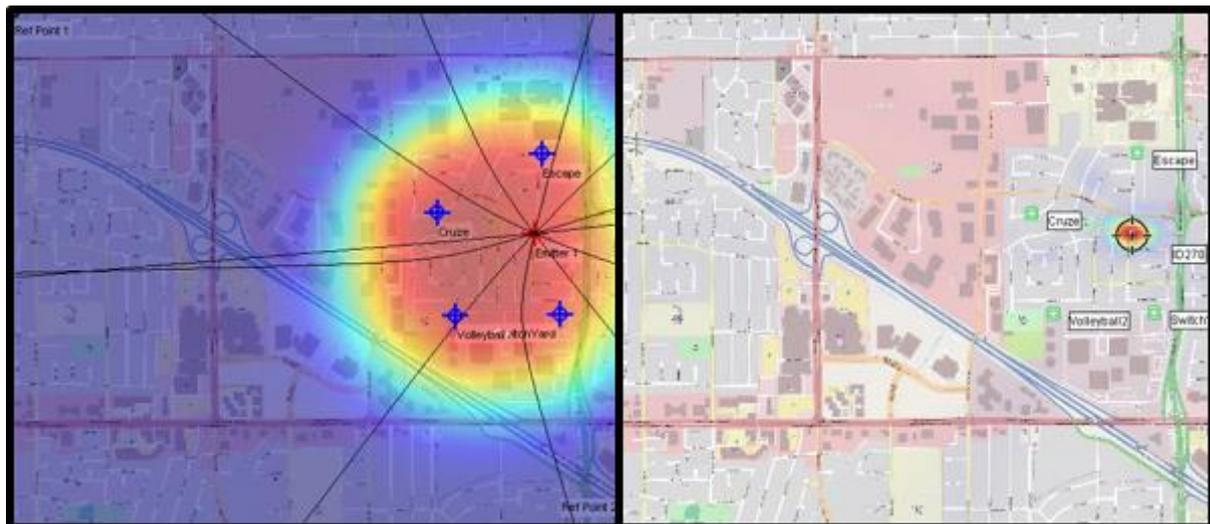
Figure 16 displays several geolocation results overlaid onto Google Earth ® with associated colorization of the likelihood, elliptical error probability (EEP) and estimated emitter position (EP). The yellow pin shows the actual location of the emitter.
