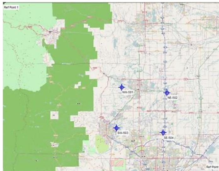
For the examples in this section, a region in the state of Colorado in the U.S. is used, as shown in Fig. 3. Four stations (NW-501, NE-502, SW-503 and SE-504) are spaced roughly 18 km apart. The simulations will illustrate RF detection range for traditional AOA and TDOA stations operating alone. For the purposes of this simulation, detection range is defined to be the furthest distance (in km) from the monitoring station that an emitter can be detected with positive SNR.
