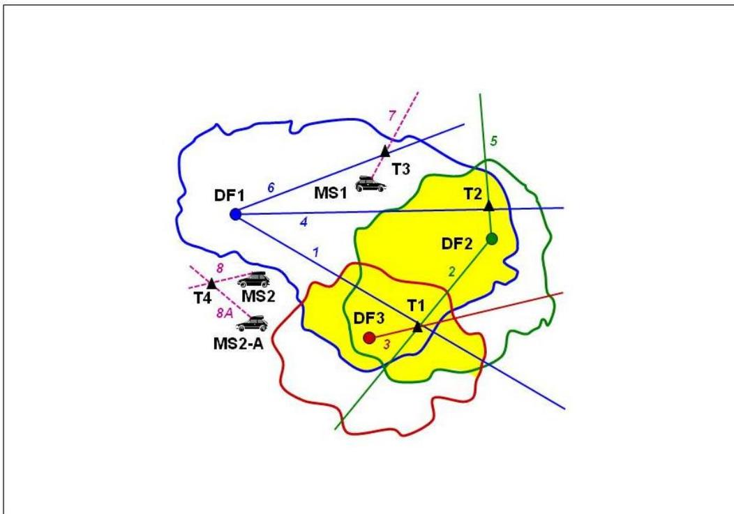
If, in a TDOA network, the transmitter of interest is situated in one of the areas outside the sensor boundary (brown colour in Fig. 1), the system may produce only one LoP, as depicted by line 2-1 in relation to transmitter T2 or a line of bearing to the transmitter. In this case, the transmitter coordinates must be determined with the help of a mobile station (MS1 in Fig. 1), interacting with the two fixed
