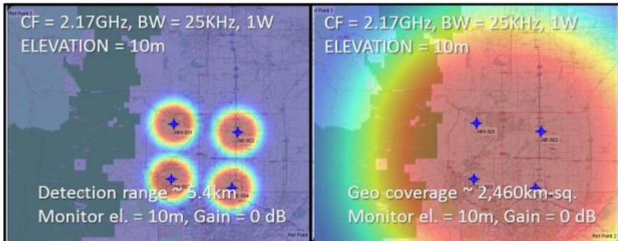
Processing gains achieved by advanced TDOA algorithms can provide emitter location capabilities over an area greater than the RF detection range of the individual stations.
