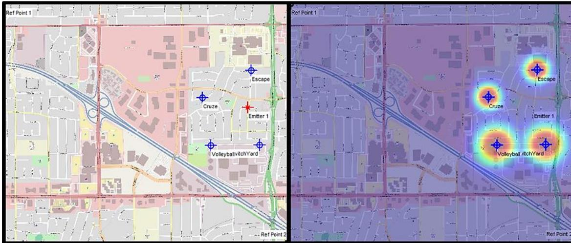
The detection range of the two southernmost monitoring stations is greater due to slightly higher elevation and directional antennas pointed north. All monitoring stations were connected via cellular modems to a geolocation server with routable IP address located in an office building in Santa Clara. Control of the sensor network was accomplished via laptop from the vehicle carrying the emitter.
