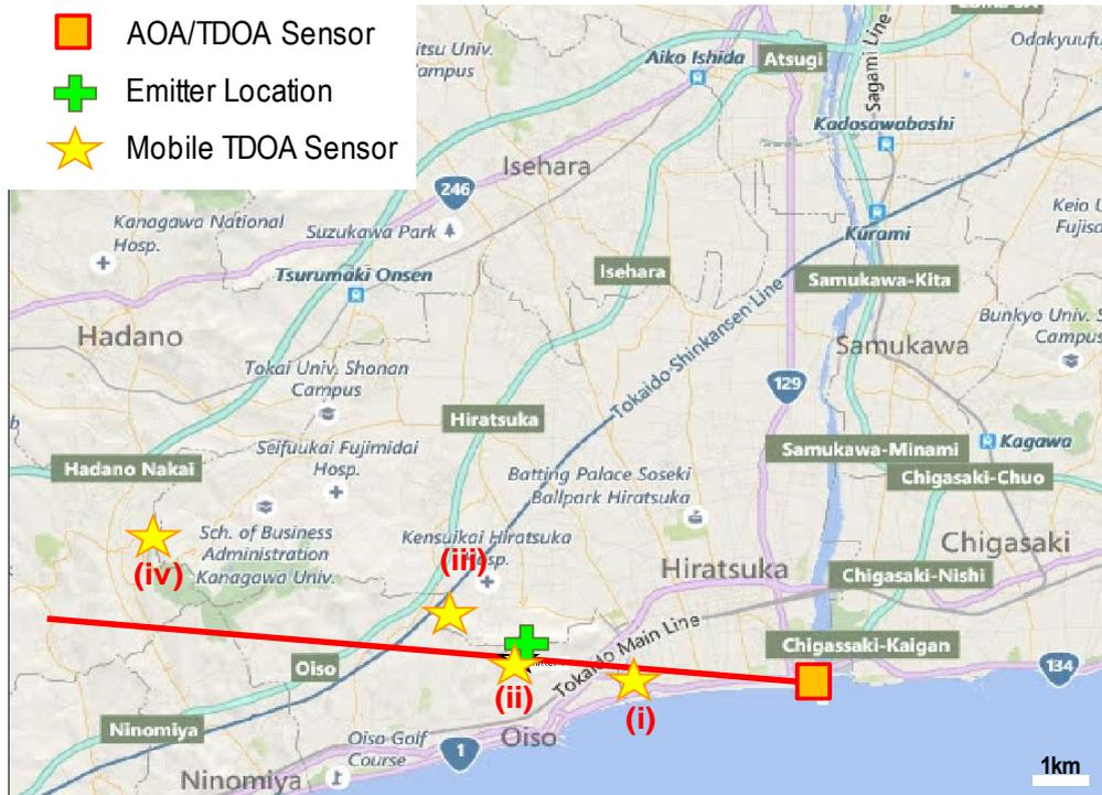
The line of bearing obtained by AOA is the red line in Fig. 22.
