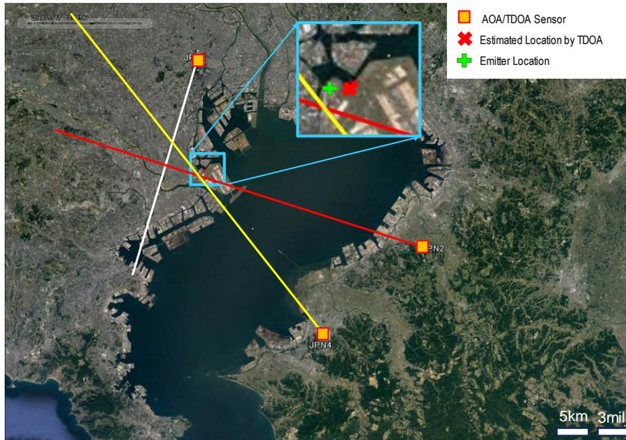
These results show that the simultaneous measurements both AOA and TDOA can reduce the ambiguity and/or improve the accuracy of emitter location measurements.
