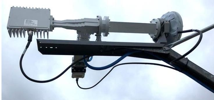
*Note to Fig. 1:* Shown in the picture are the feed, a transmit reject filter, an OMT, a solid-state power amplifier (SSPA) and an LNB. The output from the LNB and the input to the SSPA are L-band signals.
