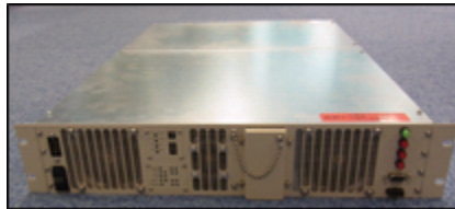
(a) Picture of the prototype modem with hardware implementation of DSDT
