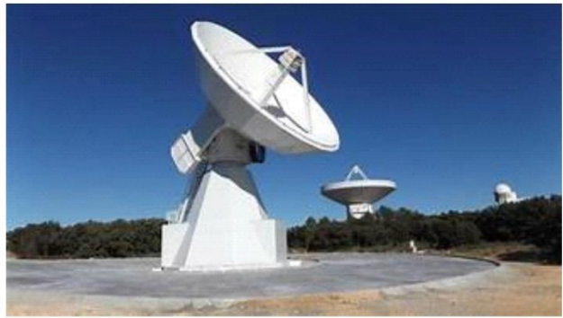
FIGURE 9 Radio telescopes used for geodetic VLBI
