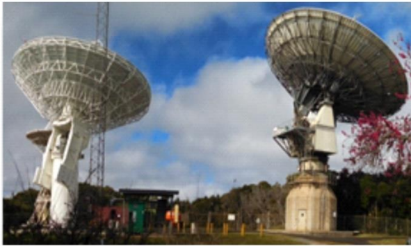
FIGURE 9 Radio telescopes used for geodetic VLBI
