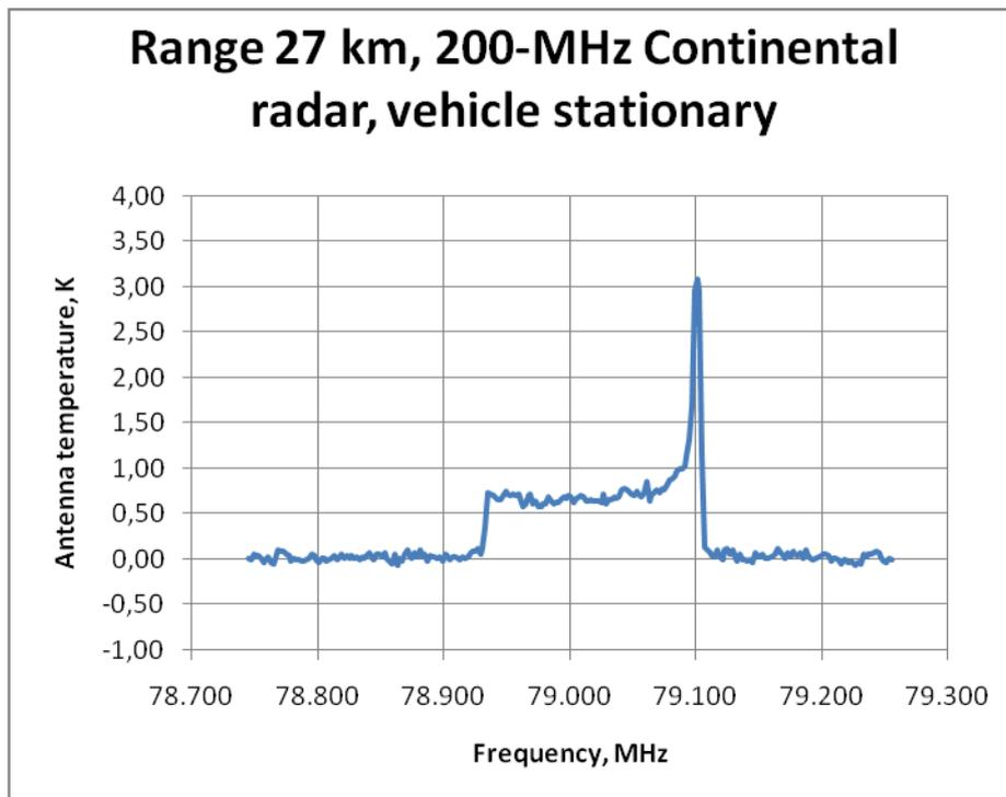
Figure 12, with the vehicle at 26.9 km and stationary, the received spfd of the plateau of emission is  $-146.7 \text{ dBW/m}^2/\text{Hz}$ ; the spike of emission is some 6.6 dB stronger. The received pfd of the plateau
