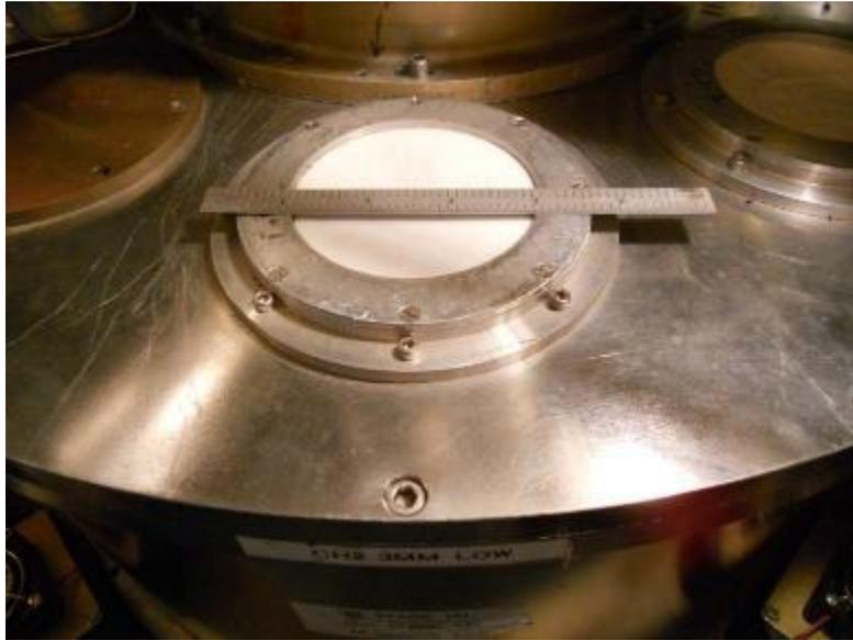
The window above the SIS (superconductor-insulator-superconductor) mixer receiver in its Dewar is shown in Fig. 9. The receiver itself is cooled to 4 K.
