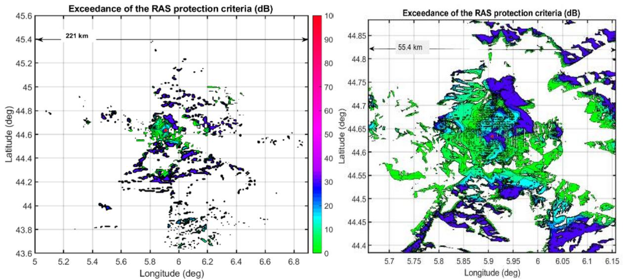
When overlapping the figure on the terrain model map, it can be seen that the results are strongly dependent on the surrounding terrain as shown in Fig. 3. These results confirm the findings from Report ITU-R M.2322 that concluded that the shape and dimension of the area from which an automotive radar could create detrimental interference to a RAS station largely depends on the terrain surrounding the RAS site.
