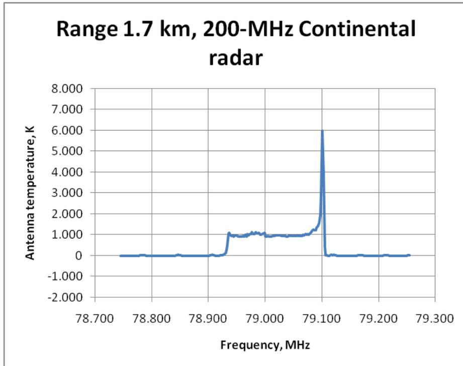
Away from the main emission of the transmitter, say  $\pm 150$  MHz in Fig. 10, there is some residual response, but at a much lower amplitude of about 11 K. This is some 27 dB down on the peak emission of 5 892 K. The theoretical rms receiver noise fluctuations for this observation are only  $\sim 0.084$  K.
