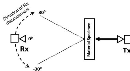
(b) Principle of reflection measurement
