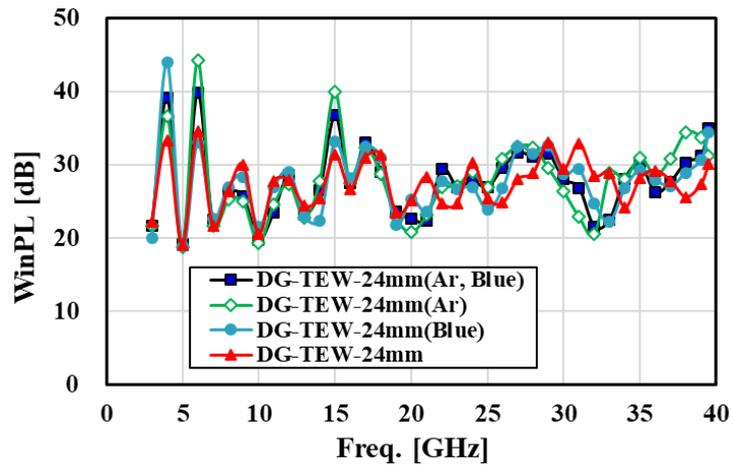
Figure 14 compares WinPL characteristics according to the type of gas in the space and window colour. Compared to a 24 mm double-glazed window (DG-TE-24mm) made of transparent glass with metal coating and filled with dry air, there is no significant difference in WinPL characteristics whether the space is filled with argon gas (Ar) instead of air or in the case of blue glass (Blue).
