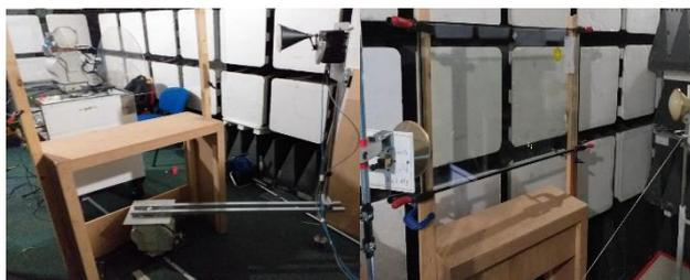
A sample of double-glazed window with a width of 1 000 mm and length of 600 mm was added for the reflection loss measurements. To perform the reflection measurements a sheet of aluminium was taken as a reference (considered a total reflector). The measurements were conducted (in co-polar (VV) and cross-polar (HV) antenna alignment) with the aluminium first (PRref) then replaced by the
