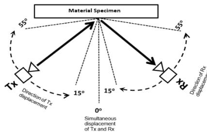
(c) Measurement setup in anechoic chamber
