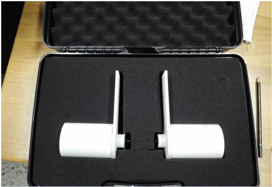
FIGURE 220 1.6 GHz~50 GHz Ultra wideband Omni-directional antennas, linear polarization
