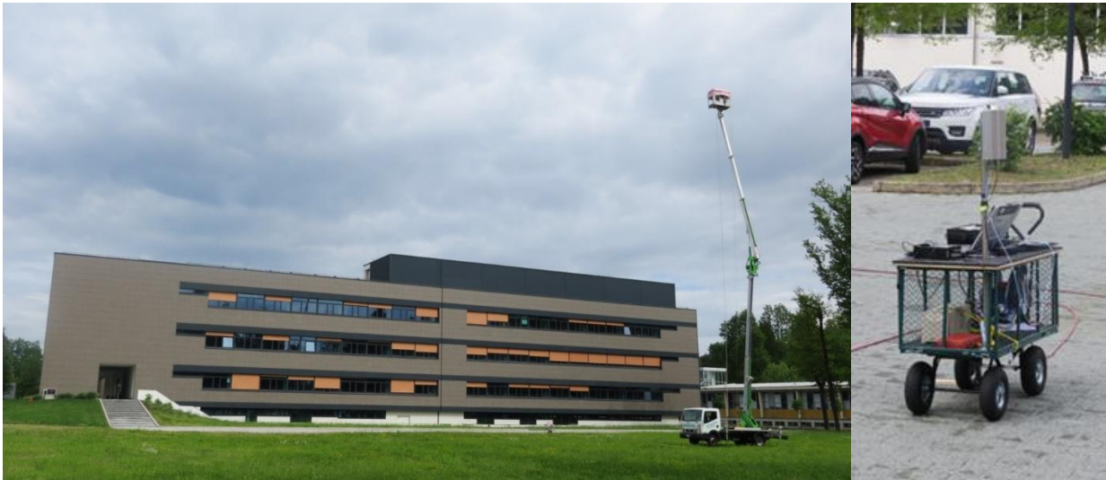
FIGURE 355 Tx on cherry picker and receiver on the trolley
