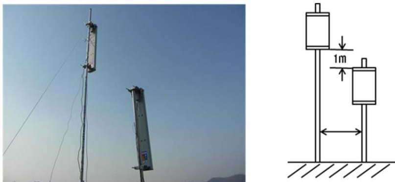
FIGURE 27 Antenna configuration for horizontal and vertical separation
