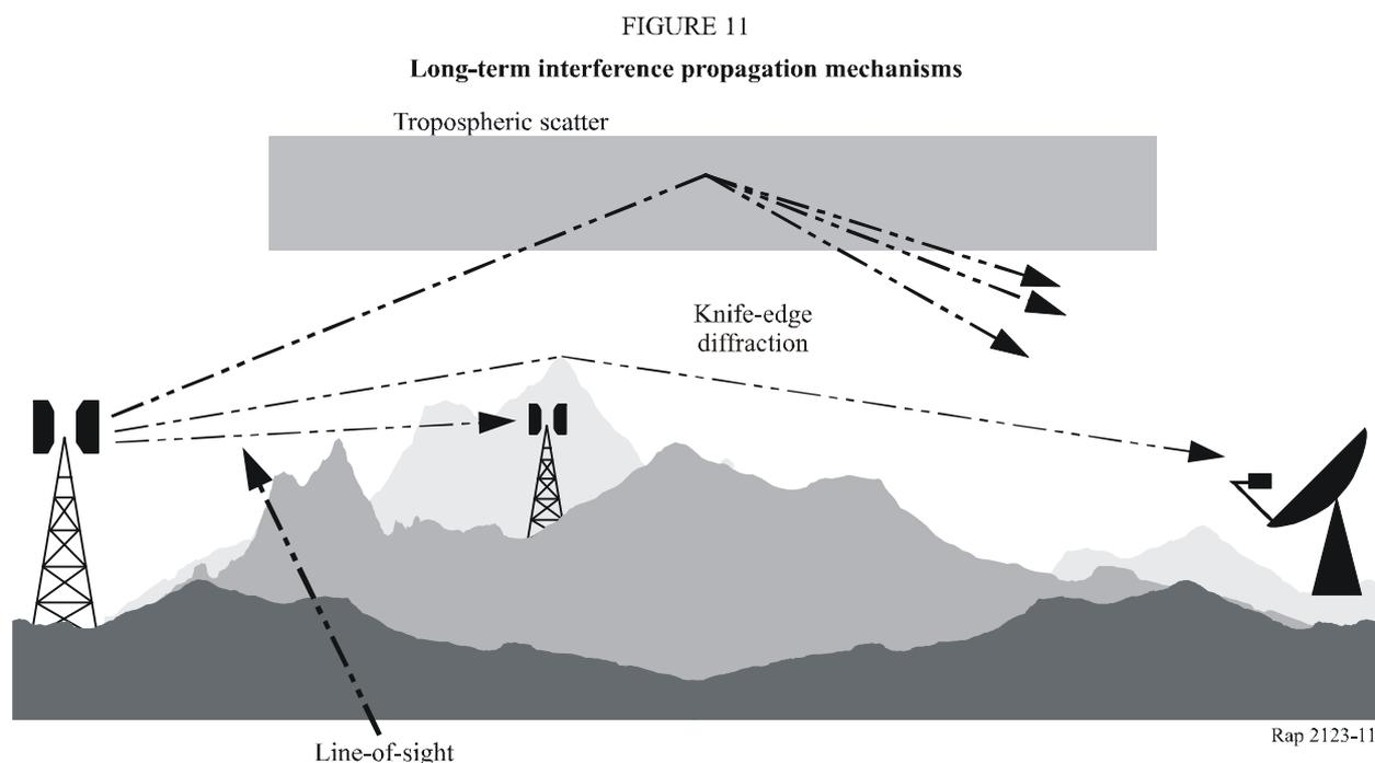
Two Recommendations of the ITU-R, Recommendations ITU-R P.452 and ITU-R P.617, provide long term statistical equations for predicting the tropospheric scatter propagation loss under various conditions. Because of some frequency limitations on these models, a third model was also investigated. The results of the investigation of these three models are discussed below.
