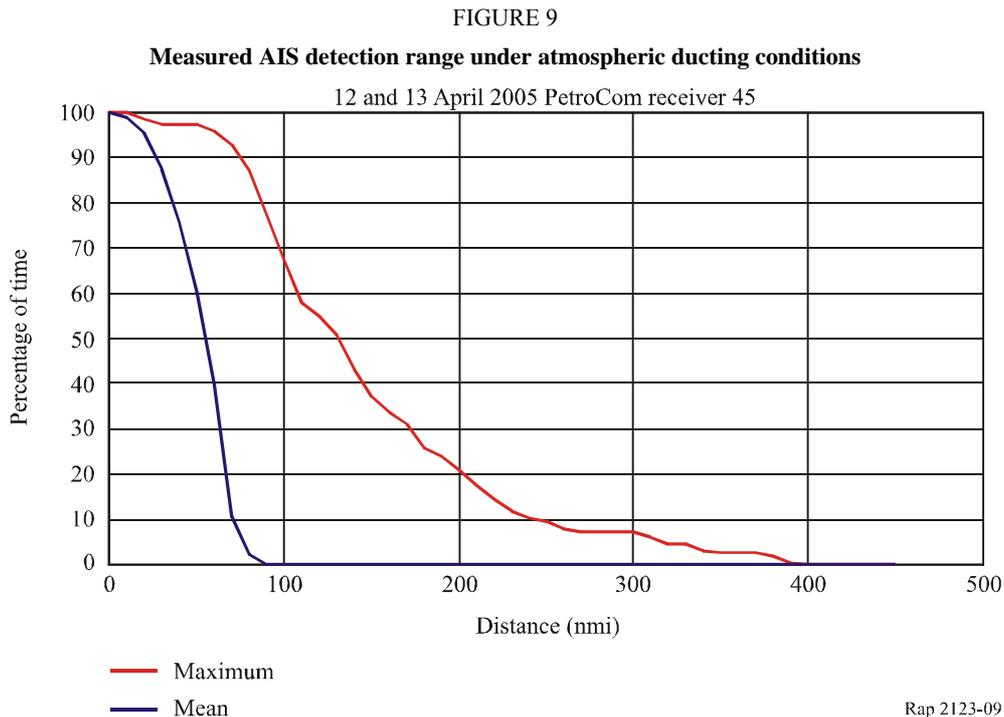
These limited measurements show that AIS detection ranges can expand many-fold during periods of atmospheric ducting.
