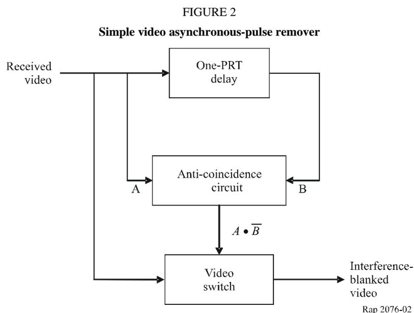
When MTI processing is performed, the problem arises that each isolated asynchronous pulse generates several synchronous pulses, with more synchronous pulses being generated when recursive or feedback cancellers are used than when only feed-forward cancellers are used. Even in the absence of MTI processing, feedback integrators can create the same problem. Two remedies naturally suggest themselves:
