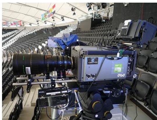
FIGURE 6 1.25-inch 4-CMOS camera and 5x lens
