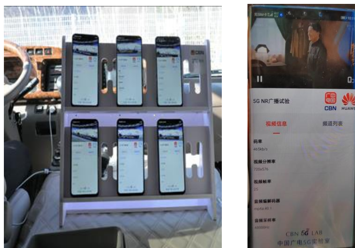
FIGURE 11 Test cells phone in test vehicle
