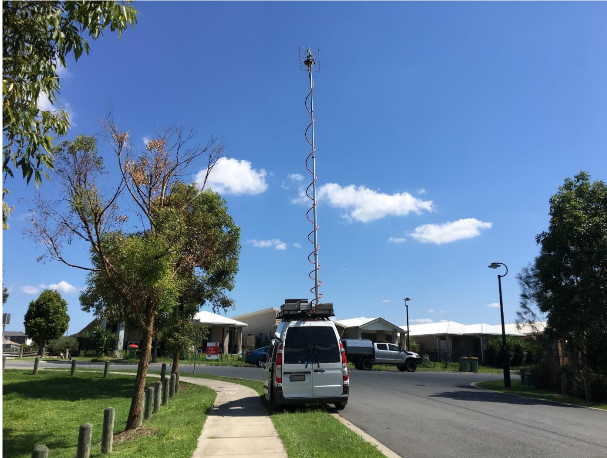
FIGURE 3-24 Extended SFN survey vehicle
