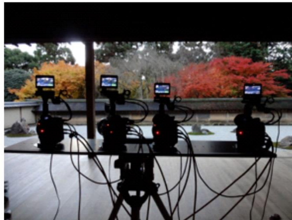
FIGURE 15 Camera array consisting of four 4K cameras
