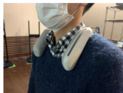
(c) Second sound device (wearable neck loudspeaker system)
