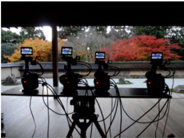
FIGURE 15 Camera array consisting of four 4K cameras
